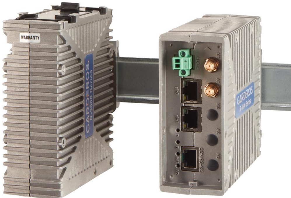
Fig. 1: Garderos R-3600 single radio routers optimized for smart grid.
